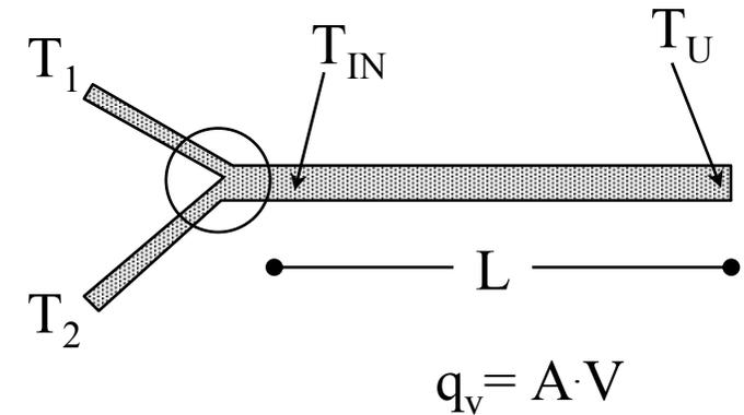
$$T_U(t) = T_{\text{IN}}\left(t - \frac{L \cdot A}{q_V}\right)$$
